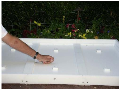
4. Using one of the “Module Attaching Screws”, attach the back side of the Center Module to the back side of the Right Module. This screw is inserted at an angle into the pre-drilled hole in the Center Module.
