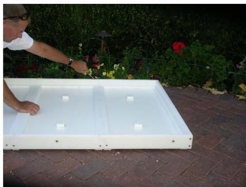
5. Then using a second “Module Attaching Screw”, attach the front side of the Center module to the front side of the Right Module.
