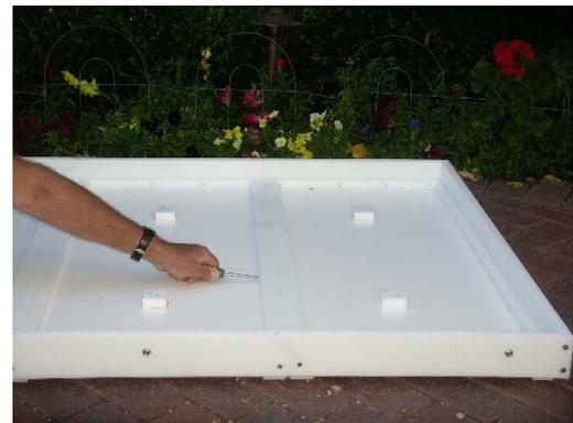
3. Then slide the Left Module toward the Center Module and attach the Center Module to the Left Module by inserting the four remaining “Center Brace Screws” into the pre-drilled screw holes.
