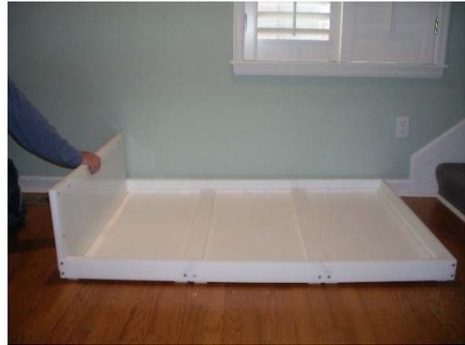
2. While holding this panel in place, slide "Panel 2" onto the left half of the back side of the box frame
