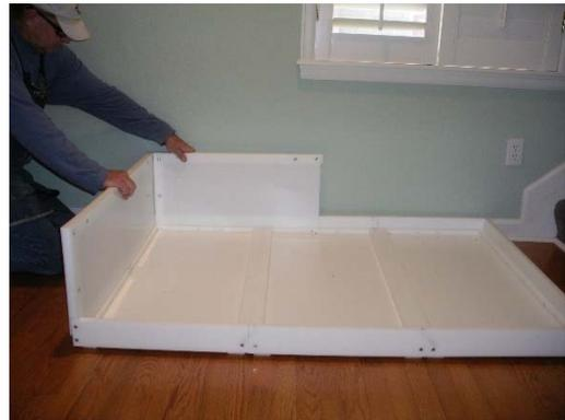
3. Take two of the "Side Panel Screws" provided and screw the back pole of "Panel 1" to the left pole of "Panel 2" using the pre-drilled screw holes.
