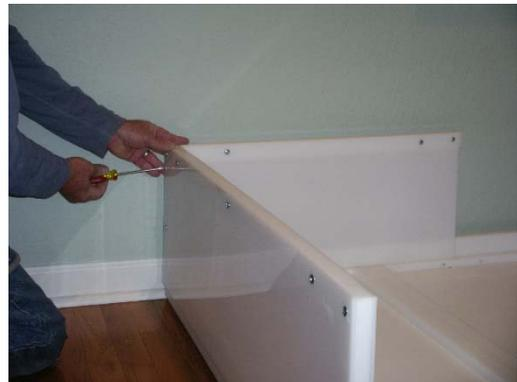
4. Position the "Back Side Brace" so that the two grooves on the left side of the brace fit snugly into the two pieces of polyethylene on "Panel 2".
