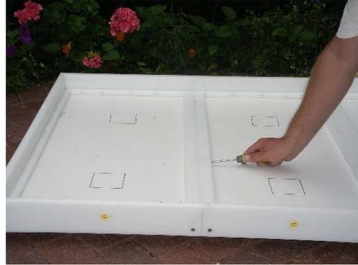
4. Using one of the "Module Attaching Screws", attach the back side of the Center Module to the back side of the Right Module. This screw is inserted at an angle into the pre-drilled hole in the Center Module. Then using a second "Module Attaching Screw", attach the front side of the Center module to the front side of the Right Module.
