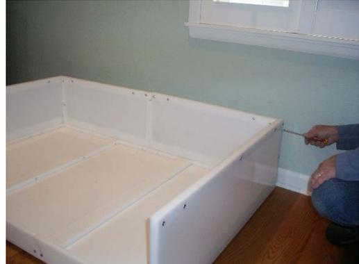
8. Using the "Base Screws" provided, attach the bottom of each of the polyethylene panels to the box frame using the pre-drilled screw holes. There are two screws for each panel.
