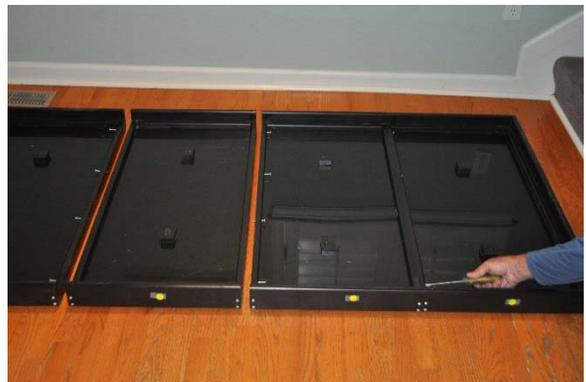
3. Then slide the Left Center Module toward the Right Center Module and attach these two modules by inserting the four more “Center Brace Screws” into the pre-drilled screw holes.
