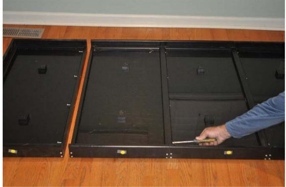
4. Finally, slide the Left Module toward the Left Center Module and attach these two modules by inserting the remaining four “Center Brace Screws” into the pre-drilled screw holes.
