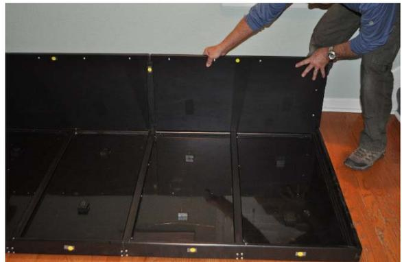
16. Slide “Panel 4” onto the right side of the box frame.
