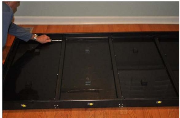
5. Using one of the “Module Attaching Screws”, attach the back side of the Right Center Module to the back side of the Right Module. This screw is inserted at an angle into the pre-drilled hole.
