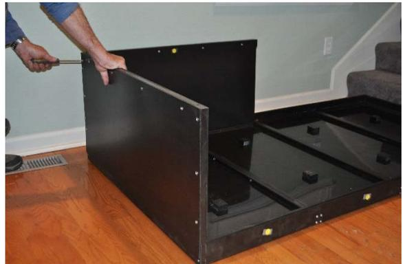
14. Position the “Back Side Brace” so that the two grooves on the left side of the brace fit snugly into the two pieces of polyethylene on “Panel 2”. The top frame of “Panel 2” should rest on top of the brace.
