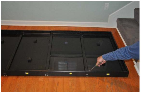
7. In a similar fashion, use the remaining “Module Attaching Screws” to attach the two center modules and the Left Center and Left modules.
