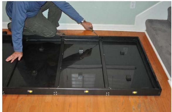
6. Then using a second “Module Attaching Screw”, attach the front side of the Right Module to the front side of the Right Center Module.
