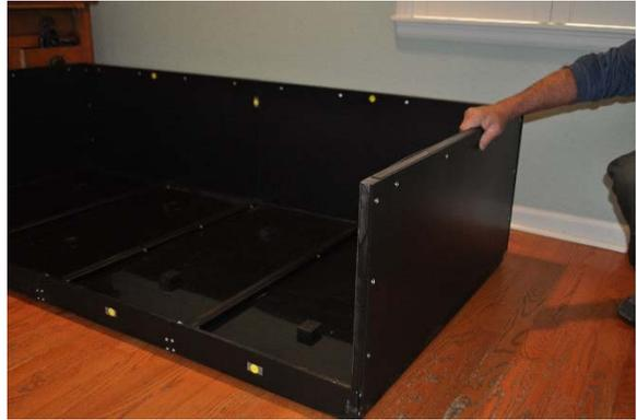
17. Use the remaining two “Side Panel Screws” to screw the back pole of “Panel 4” to the right pole of “Panel 3” using the pre-drilled screw holes.
